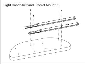
NOTE: The Half Moon Lazy Susan ships ready to install as a Left Hand model. Apply first set of screws on A,B or C when converting to Right Hand model. Attach second set of screws where they are positioned.
