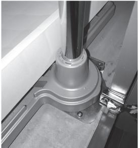
Place one of the Shelf Assemblies on top of the Lower Hub Assembly and secure in position by sliding the pole through the center, pushing firmly until the pole is at the bottom of the cabinet.
