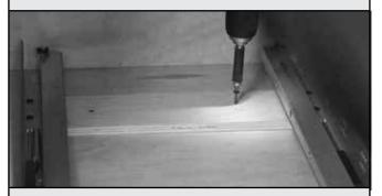
Secure the base unit by screwing through the plywood runners (front & back) with the (4) #8 x 1" coarse-thread wood screws provided.
