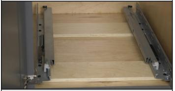
Place the base unit inside the cabinet. Position it left to right, ensuring proper clearance for hinge or door protrusion.
